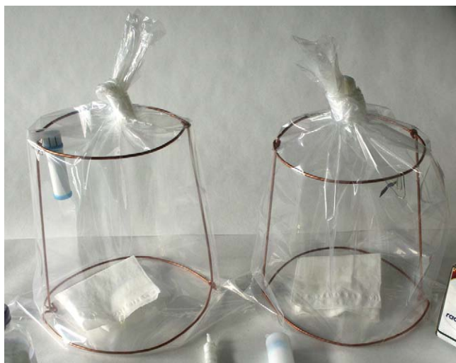
Fig. 2. Passive headspace extraction preparation with a Radiello device (left) and an activated carbon strip (right).
